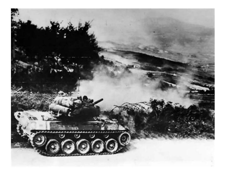
While tanks were crucial, tank destroyers played an equally vital role in the United States' armored forces. The M18 Hellcat emerged as one of the most successful tank destroyers of the war. With its exceptional speed, it could outmaneuver enemy tanks and strike with lethal precision. Its thin armor belied its deadly capabilities - the Hellcat was armed with a 76mm gun, capable of taking out even the most heavily armored adversaries.
