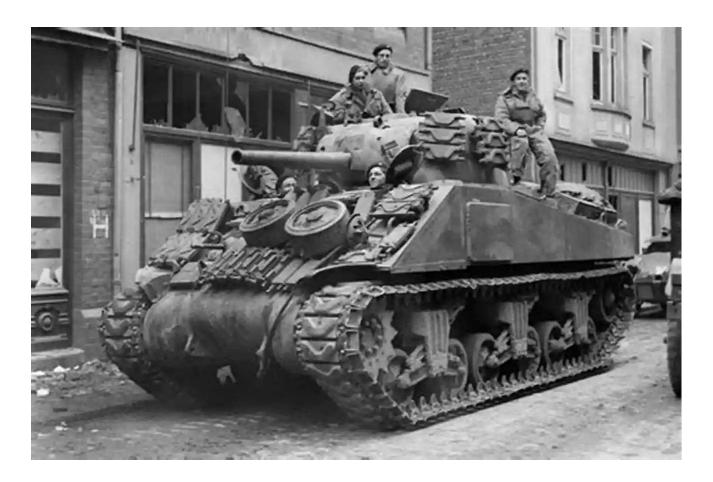
One tank that stood out in the American arsenal was the M4 Sherman. With its distinctive shape and robust construction, the Sherman became synonymous with American armor. The M4 Sherman boasted a 75mm gun, which enabled it to engage enemy tanks effectively. Its adaptability and maintainability made it a mainstay on the battlefield, providing American forces with the needed firepower and mobility to outmatch their adversaries.
