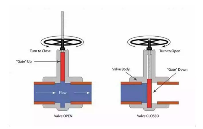
Gate valves are widely used in the oil and gas industry, as well as in water treatment plants. They are designed to provide a straight-through, unobstructed flow path by using a gate or wedge-shaped disk.
