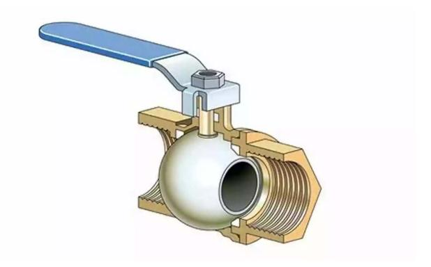
Ball valves are known for their durability and efficient performance. They consist of a ball-shaped disk with a hole in the middle, which rotates to control the flow.
