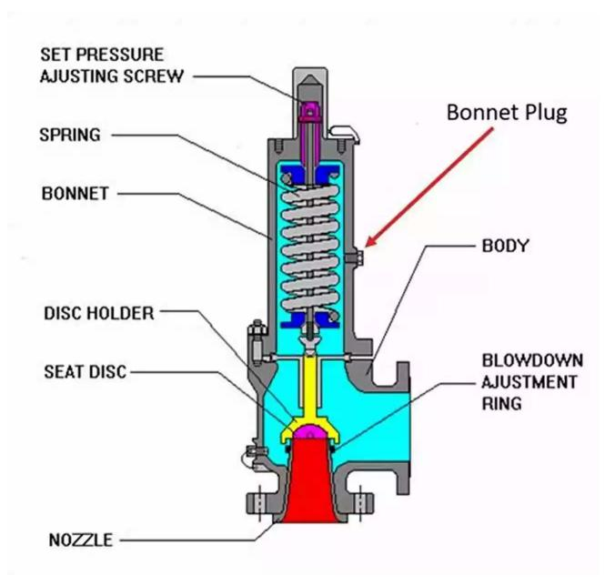
Pressure relief valves are vital for maintaining system safety by preventing excessive pressure build-up. They open automatically when the system pressure exceeds a set limit, releasing the excess pressure.
