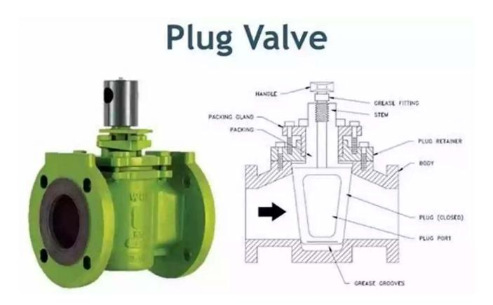
Plug valves consist of a cylindrical or tapered plug with a hole passing through it, enabling control of the flow by rotating the plug. They offer high reliability and easy maintenance.
