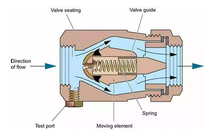
Check valves are designed to prevent backflow in a pipe system. They allow flow in one direction while blocking any reversal, ensuring the protection of equipment and preventing process interference.
