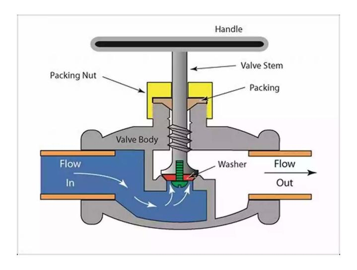
Globe valves offer excellent control and throttling capabilities due to their versatile design. They have a disk that moves perpendicular to the flow direction, allowing precise regulation of fluid flow.
